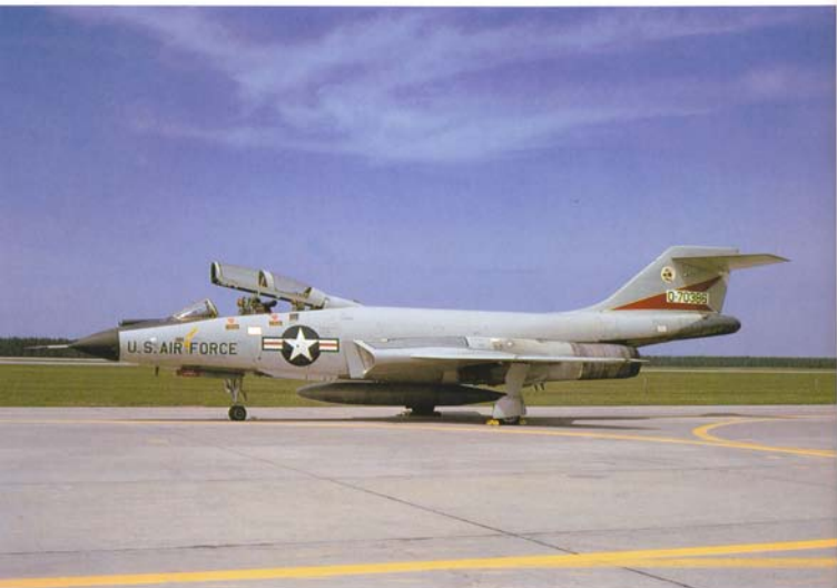
Above The infrared sensor forward of the windshield replaced the retractable inflight refuelling probe initially fitted to Voodoo interceptors. With its large clamshell canopy open, this TF-101F-96-MC of the 62nd FIS at KI Sawyer AFB, Michigan, clearly shows the sun shield mounted over the radar scope in the rear cockpit
