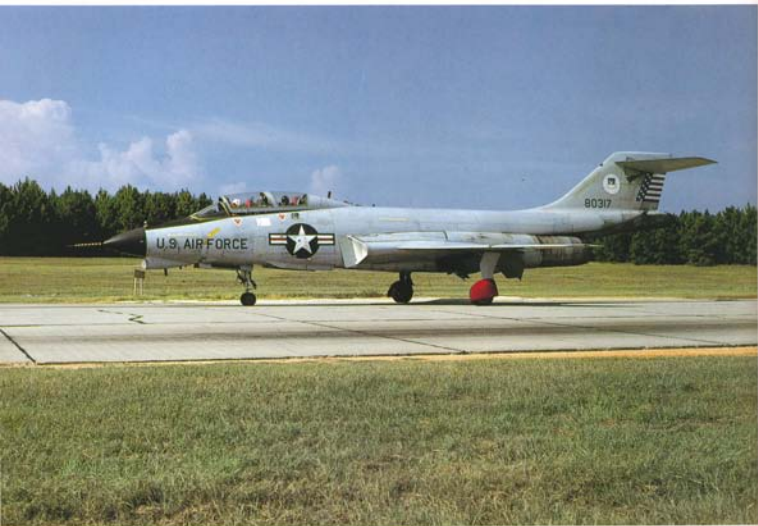
Above Photographed at Tyndall AFB on 25 September 1978, this Voodoo of the 2nd FITS was fitted with an experimental sensor in a fairing beneath the nose cone
